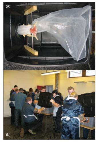
**Figure 7.** The ewe simulator (a) top view showing 'uterus' (b) first year students practising on the simulators Photo credits: Isobel Vincent, RVC
