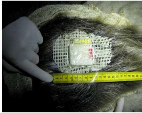
Figure 49. GPS and VHF tag on mesh, glued to adult beaver's back (SBT).
