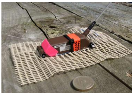
Figure 46. Metal-encased ARGOS satellite tag. Figure 47. Reinforced plastic-encased RF tag on mesh (SBT).
