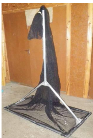
Figures 29 & 30. A specially-designed beaver landing net (SBT). Net frame should be around 100 x 85cm and attached to a ~200cm long iron/aluminium tube. The frame can rectangular or more oval/circle shaped. Joints should be strengthened for durability.
