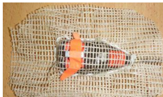
Figure 46. Metal-encased ARGOS satellite tag. Figure 47. Reinforced plastic-encased RF tag on mesh (SBT).
