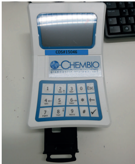
Fig 5: Dual Path Platform (DPP) VetTB test electronic reader provides a semi-quantitative measure of the antibody response in a given serum sample. Picture: Sandrine Lesellier, APHA
