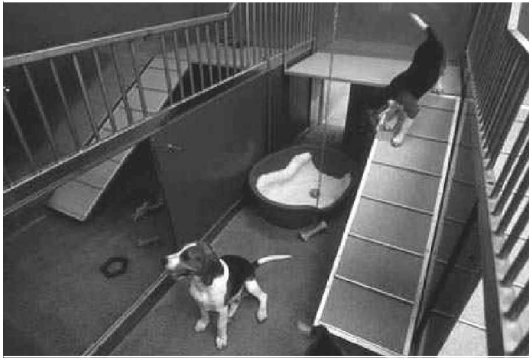
Fig 10 Dog pens designed to meet the behavioural needs of the dog. The pens are linked in pairs with access to an outdoor area through the pop-hole at the back of the pen. Pen subdivisions allow complexity and choice. Raised platforms offer visibility across the room. Suspended chews are provided as means of environmental enrichment. A dog bed with fleecy bedding offers a comfortable resting place
